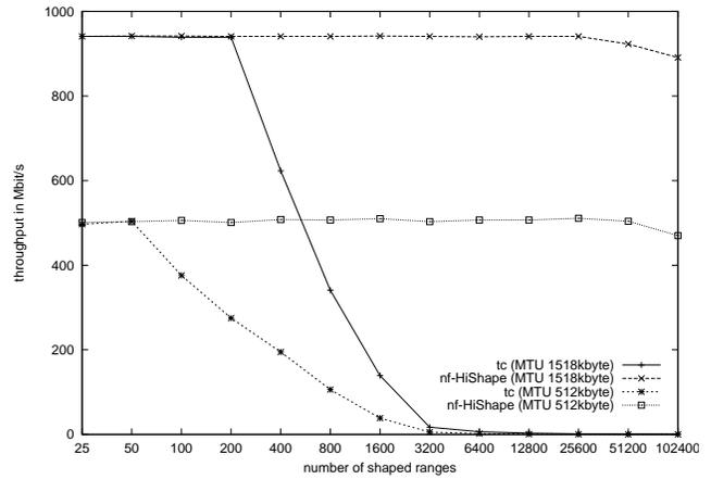
**Figure 1:** *nf-HiShape* is able to handle more traffic than *tc* on large sets of shaping rules
